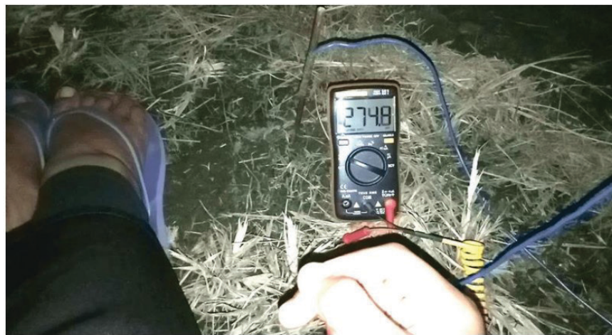
Figure 3. In an experiment measuring skin voltage when not grounded/not Earthing, a skin voltage of 274.8 millivolts
