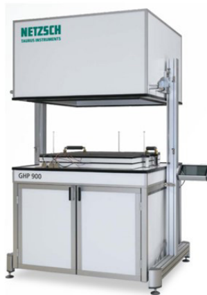
Gambar 2. GHP 900 – Thermal Conductivity Tester
